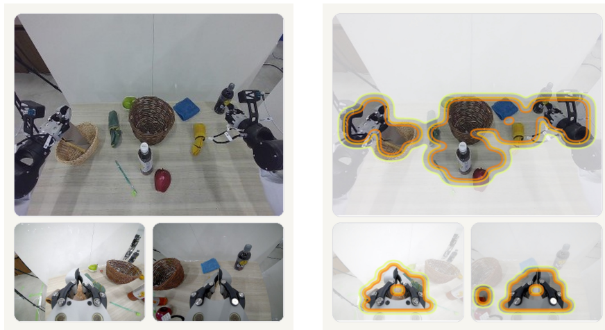
Figure 10 | Representative cluttered TX-G2 observation (left) and the corresponding S2 mask (right) for the ordered clothes-sorting task. The tabletop contains many distractors absent from the training set, yet the learned mask remains concentrated on the task-relevant garment, end-effector, and basket region.
