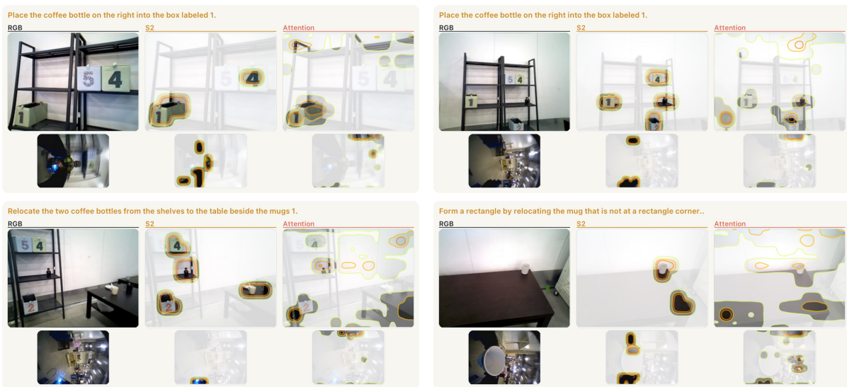
Figure 9 | Additional real-robot qualitative comparisons between the learned visual evidence budget and the backbone’s native attention. Each panel shows the RGB observation, the learned S2 mask, and the corresponding \pi_{0.5} attention map for the same state. Across both TX-G2 and HSR, VEB remains more concentrated on the object, contact region, and target placement context relevant to the current behavior, while native attention is often more diffuse.
